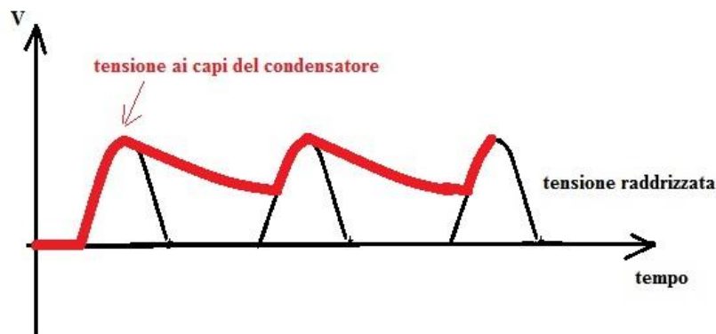
Figure 16 Filtered single wave rectifier waves
